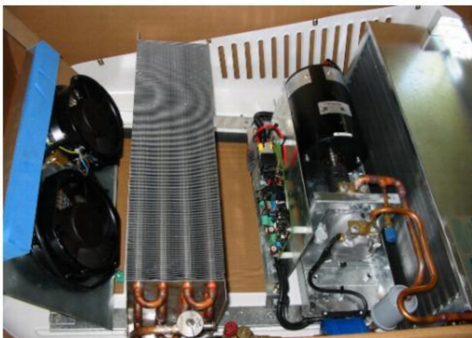
40 cc Rotary Compressor & DC Electric motor with direct drive set-up
