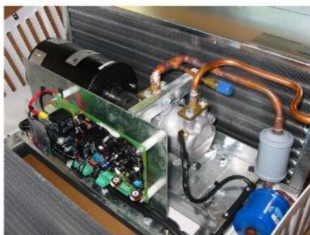
40 cc Rotary Compressor & DC Electric motor with direct drive set-up
